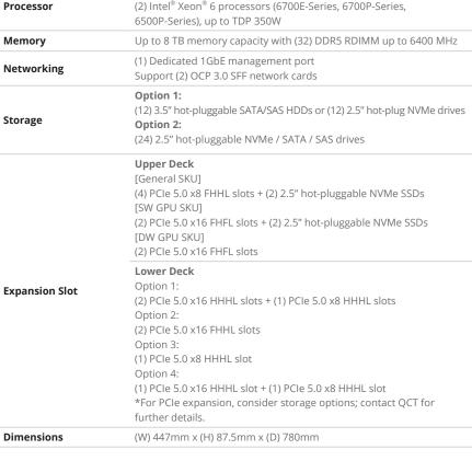
server equipped with dual Intel<sup>®</sup> Xeon<sup>®</sup> 6 processors, 32x DDR5 RDIMM memory of up to 6,400 MHz, and versatile storage options including 3.5" and 2.5" drives. It features flexible networking with 2x OCP 3.0 SFF slots and offers multiple PCIe 5.0 expansion options, making it a versatile solution for diverse device support in modern data centers.
