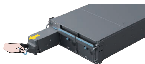
Pump Filter Module
