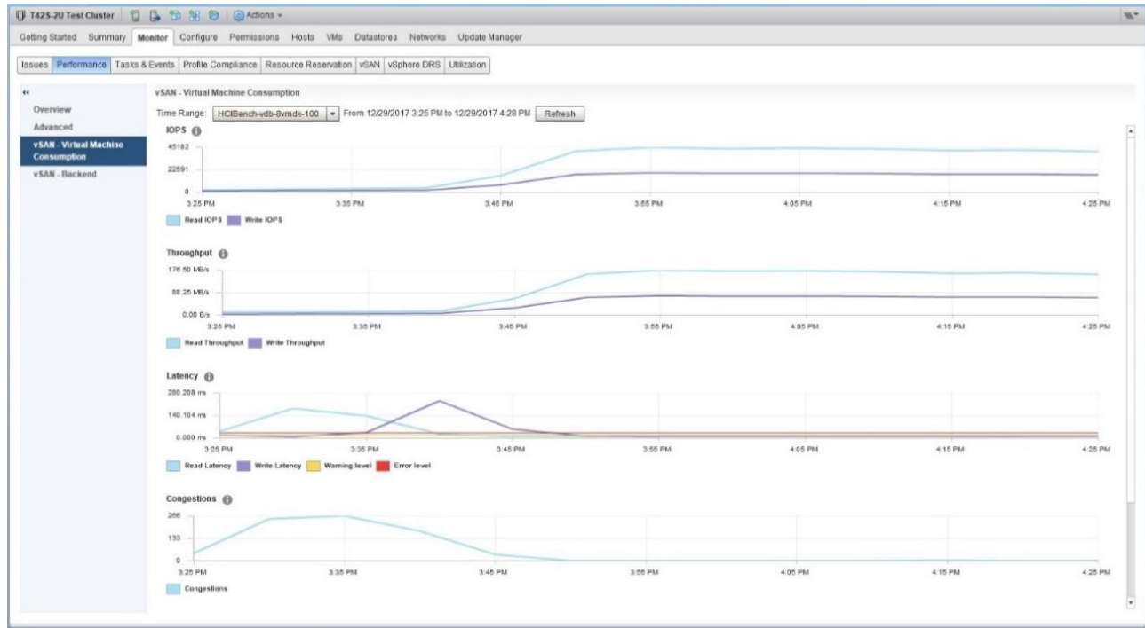
Figure 21. Graphical Results of IOPS, Throughput, and Latency for Test Case 3.
