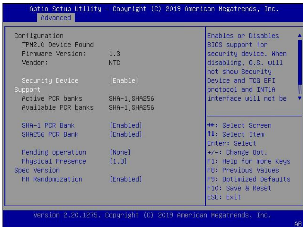
Figure 8. Discovery of TPM 2.0 device in BIOS.
