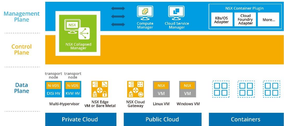
Figure 1. NSX-T three plane architecture.
